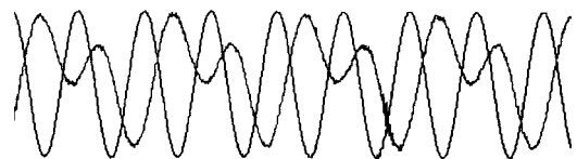
FIG. 4. Supply voltage ( \nu_0 = 473 kHz) and received signal (containing harmonics) as a function of time. Arbitrary ordinate scales.
